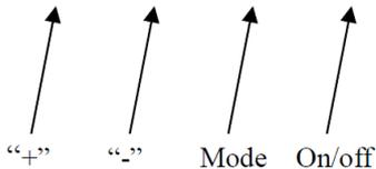
⏻ Press this button to power on the LCD display, Long pressing the button for 2 seconds to power off. Automatically shut off without any operation in 5 minutes.
