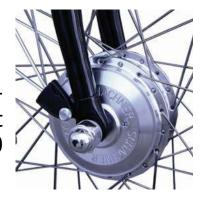
The motor is mounted in the fork with two nuts and secured with two safe holders. If you want to remove the motor from the bike, for example if you want to change the tyre, please take car that you insert the motor in the right position again and that the cables are not damaged.
