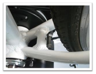
For the safety of the frame the clamp can be covered with a shrink tube. (not included in the scope of supply)
