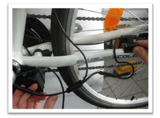
Now the battery can be inserted and the kit is fully assembled.
