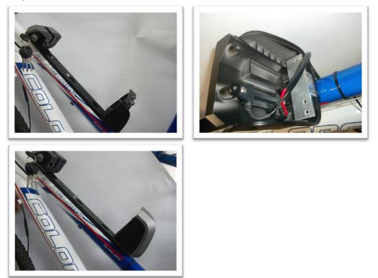
Screw the cover with the 4 tappings screws.
