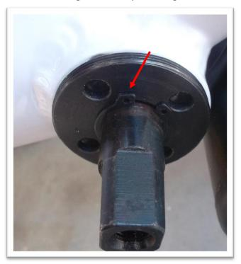
Now plug the magnetic disc on the axle. Make sure that the magnetic disc is free to rotate on the axle!
