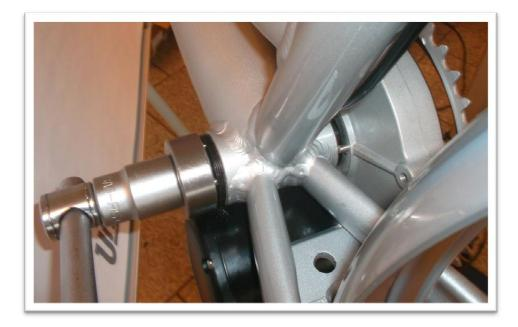
Loosen the screws and remove the motor again!
