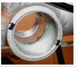
Draw on the depth of the recess next. This should be 5mm!
