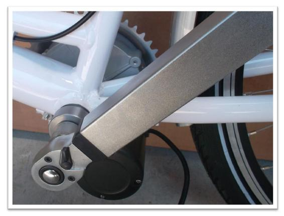
Pull the mounting tube with a torque of 85Nm fixed!
