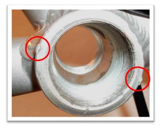
Draw on the size of the recess. This should be 5mm!
