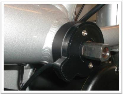
Now mount the sensor with the two M3 screws for the pedal sensor.
